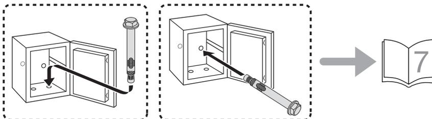
GB The safe must be anchored before being use.
