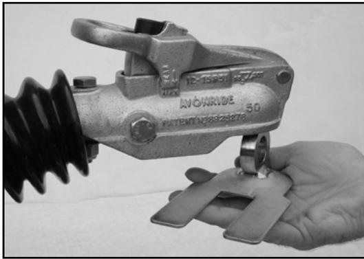
1. Insert dummy ring plate when trailer is unhitched by offering up at an angle and twisting into place.
