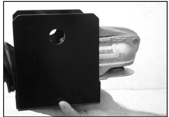
2. Offer up bottom channel according to your hitch type. Short fill strip at front for 12 - 14304 or tall fill in strip at front for standard hitch head.
